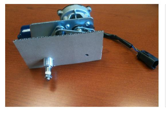
Assuming that the cardboard is the metal skin of the cab, pass the pivot shaft through the large hole from the inside of the cab. Position the mounting hole of the motor bracket with the hole in cab.
