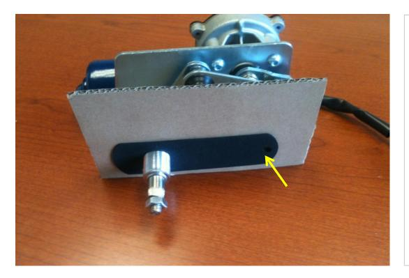
Slide the GS01550001 gasket into position, as shown. This gasket provides a snug fit between the adapter and the cab. Align the M6 hole carefully.
