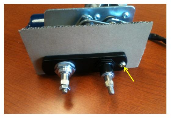
Install the WA10655001 lock washer on the 106801 bolt, and thread it through the adapter plate, the gasket, and into the motor bracket.
