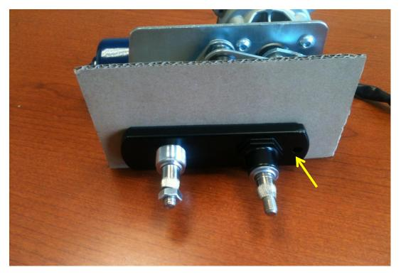
Slide the SP20260002 slave pivot adapter into position, over the gasket, as shown, taking care to align the 6mm hole on the adapter with the corresponding hole in the adapter, and the corresponding hole on the baracket.
