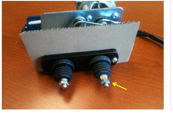
Install the WA40805001 wavy washer, and NT00800001 M8 nut onto the slave pivot.
