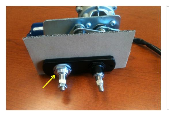
Re-attach the 20mm washer and 20mm nut that was removed from the original compact drive assembly. Do not tighten at this point.
